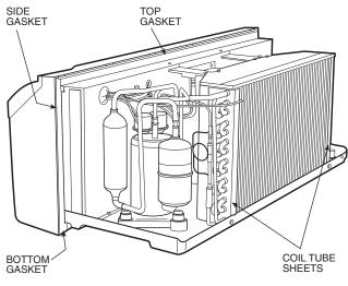
FIGURE 8 — UNIT GASKETS AND TUBE SHEETS
